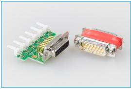
Figure 19: I1-ACL with dummy feedthrough adapter
