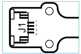
Figure 13: 4p WR-FPC 1.00mm FPC ZIF (top view)
