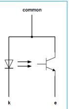
Figure 10: photo interrupter typical connection scheme
