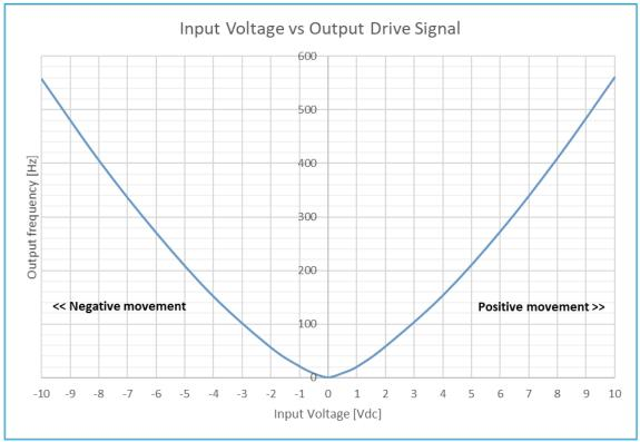
Figure 4: Input signal vs output frequency
