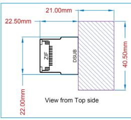
Figure 14: (approx.) Dimensions FPC to D-Sub Interface
