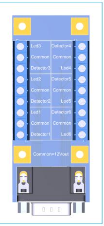
Figure 23: I1-EDM terminal board
