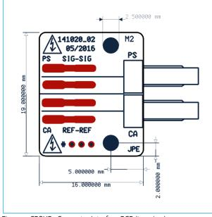
Figure 3: CPSHR1 Connector Interface PCB (top view)
