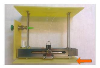
Remove the **4 threaded bars**. Again, <u>take care not to damage the fiber while using handtools to remove the bars</u>.
