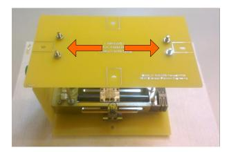
3 Remove the **bottom** Transport PCB and place the CLD on a flat surface.
