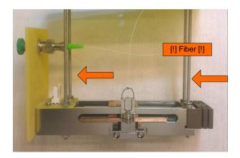
(When installing system in customer setup) Unscrew the optical fiber connector from the feedthrough that is mounted in the feedthrough PCB. Remove the feedthrough PBC from the CLD.
