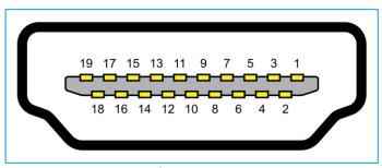
Figure 7: HDMI-type connector (front view)
