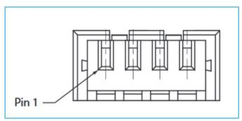
Figure 15: 4-pin WR-WTB 1.25mm Female (front view)
