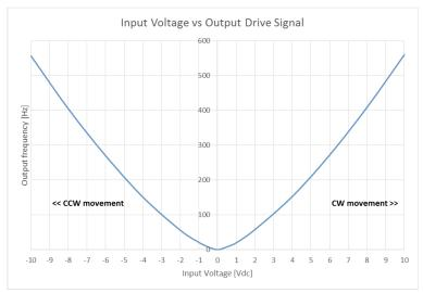
Figure 4: Input signal vs output frequency
