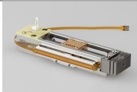
Figure 5: CLD<sub>1</sub>-RLS FPC can be seen at the back
