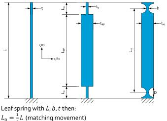
Leaf spring with L, b, t then:  $L_0 = \frac{1}{6}L$  (matching movement)  $t_0 = 0.9t$  (matching  $C_x$ )  $t_{RF} = 5t_0$  (guideline for reinforcement)  $L_H = \frac{5}{6}L$  (matching movement)  $h = \frac{1}{2}t$ D = 2h (elastic hinge guide line)  $\frac{1/1}{1}$
