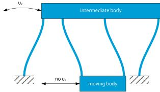
The drive stiffness ( $C_x$ ) halves; however the guiding stiffness ( $C_z$ ) halves as well.
